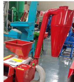
Up inlet for grain milling & cyclone for collect power
